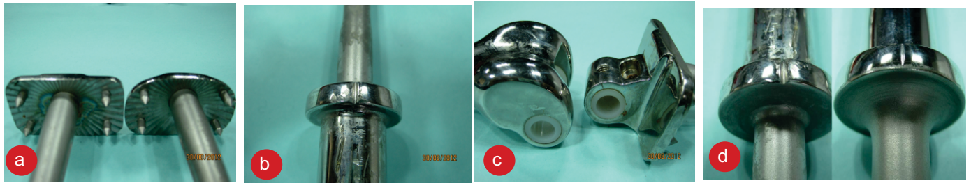
Figure 7. Changes in Tibia: a -Tibial baseplate acquired its rounded geometry conforming to the tibial plateau. b -important alignment mark on the stem was added. c -Bushes and a bumper manufactured from UHMWPE were added to minimize metal on metal articulation. d -A gradual change of diameter centered near the stem-bone junction was introduced to reduce stress concentration by introducing a fillet with a liberal radius of curvature
