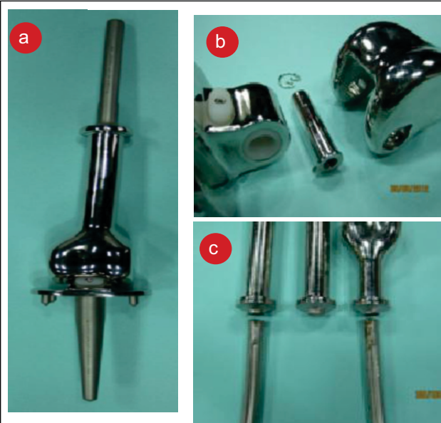
Figure 8. a , b - Standard prosthesis was almost perfect with only problem being intramedullary stems that continued to fail at the stem-bone junction ( c ) and even the reduced stress concentration with the filleted design did not seem to work
